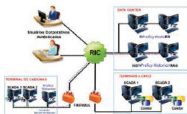
Figure 4 - InfoSCADA Project Architecture for data collection and access for corporate users
