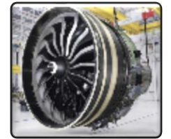
GE9X engine 10% better SFC c) compared to the GE90-115B & 5% better SFC c) than any other engine in its class
