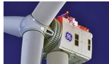
Renewable Energy's Haliade-X prototype began operating at 14 MW in Rotterdam, Netherlands
