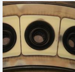
Diffusion combustors Max \text{H}_2 ~30–85%
