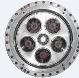
Premixed combustors Max \text{H}_2 ~20–30%
