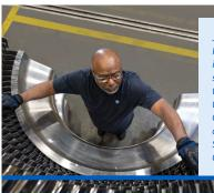
James Thomas from our Gas Power manufacturina plant in Greenville, S.C. installs a stator blade assemblu for the 7HA turbine. Two 7HA turbines along with other GE technology will help deliver up to 1,050 MW for Seminole Electric in Putnam County, Florida.
