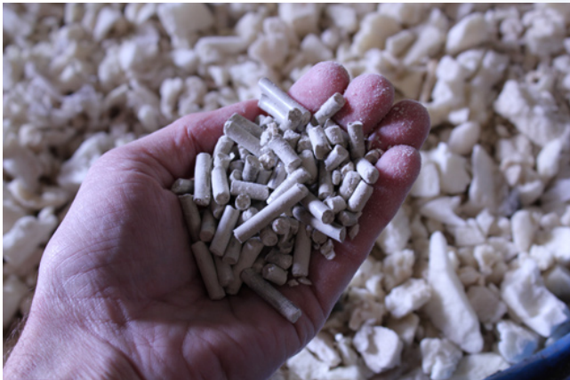
The URT system can transform refrigerator insulating foam into pellets for use as fuel or other products.
