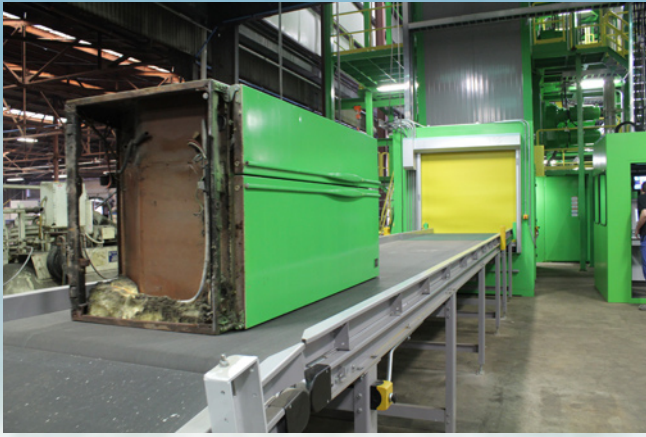
The URT system can process approximately one refrigerator per minute.
