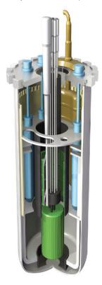
The PRISM reactor builds on sodium-cooled reactor experience and employs passive safety design features. It is a simplified reactor design, allowing factory fabrication with modular construction and ultimately lower costs.
