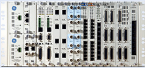
Access cross-connect multiplexer
