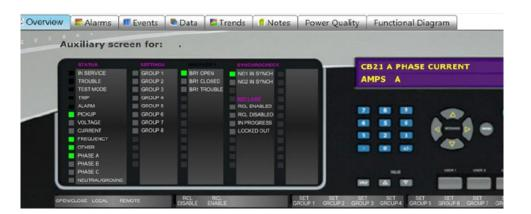
Equipment controls in iPower are provided via universal control and information containers for each device called Tab Displays. These provide convenient access to all data, controls, and user material for each device.
