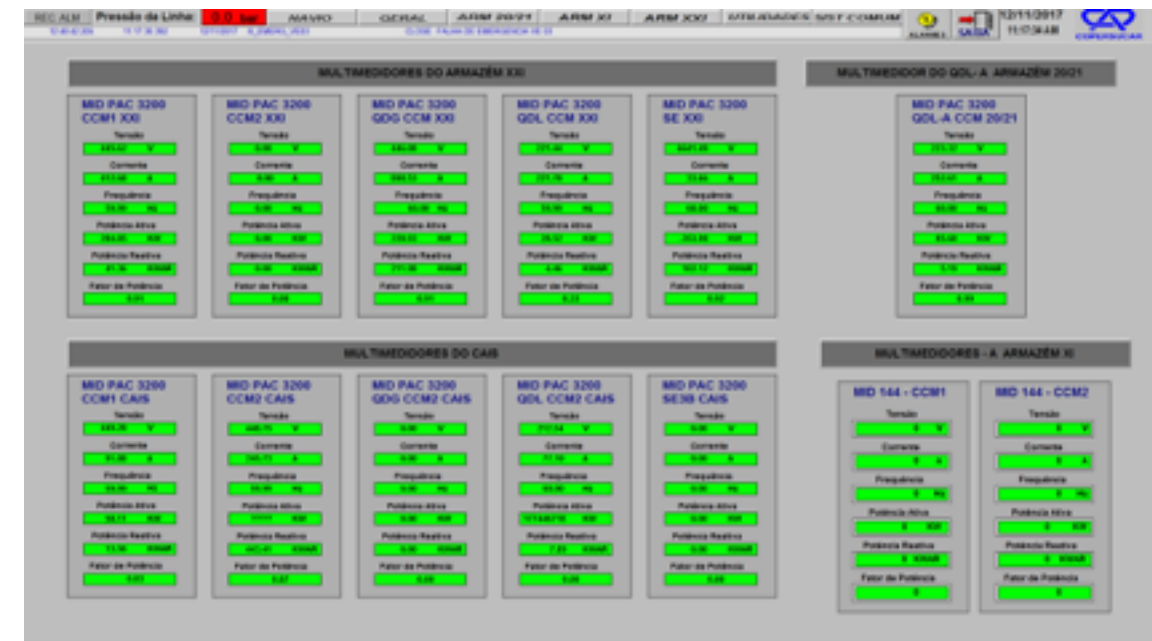
Figure 5: Electrical Quantities - Optimized on a Single Screen
