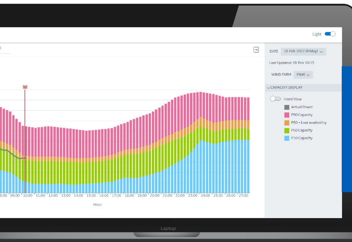
Figure 3. The GE Digital AI/ML model predicts wind turbine power generation during 15-minute intervals for the day-ahead market and displays the actual turbine farm combined output. The model also includes predicted “lost availability” based on equipment degradation. Source: GE Digital
