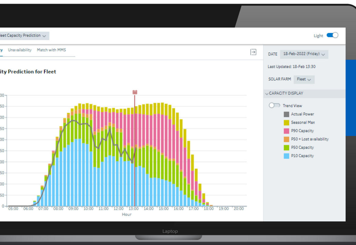
Figure 4. The GE Digital AI/ML model performance predictions for a solar field with real-time production superimposed. Source: GE Digital
