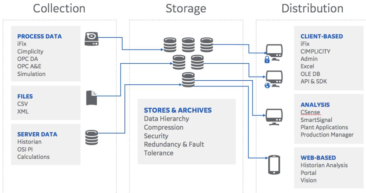
The benefits of using a system like GE Historian include recording large amounts of process data from a wide range of data sources, compressing data, and at the same time providing fast writing and reading speeds up to real-time acquisition in the microsecond range. In addition, the software's special compression algorithms enable secure data storage for years—without the need for active maintenance or back-up routines.
