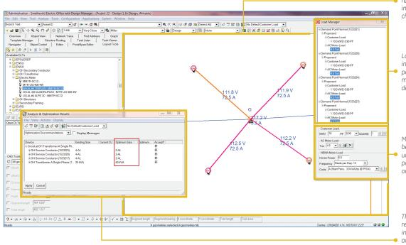
The Map window provides a highlighted thematic view of electrical analysis results during the design process indicating success or failure of designed changes.
