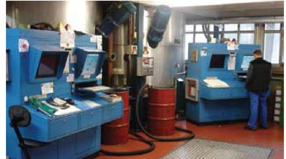
*Using CIMPLICITY, the production staff member logs his system along with the starting time and temperature onto the energy management system of the power station. After the last heating cycle of a batch, the system automatically logs off again.*
