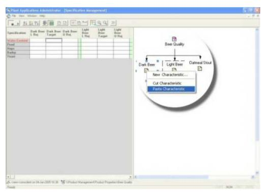
The pasted characteristic will become subordinate and any changes made to the higher-level characteristic will propagate down to the subordinate characteristic.
