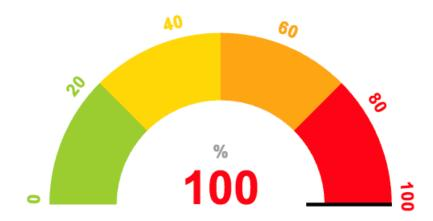
• Meter - Radial: In this gauge type, the value is plotted on a circular scale. The gauge can be an internal radial or an external radial depending on whether the scale appears inside the radial or outside. For example, the following image represents an external radial meter gauge that plots the temperature inside an engine combustion chamber.
