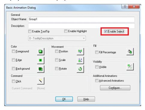
With traditional iFIX pictures, selecting the **Enable Select** property allows an object to be selected in the runtime environment.
