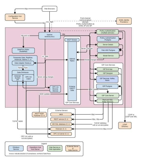
Most notable is the pink-colored box in this diagram, which represents the host where Operations Hub is deployed to – which is the trust boundary from security's point of view.
