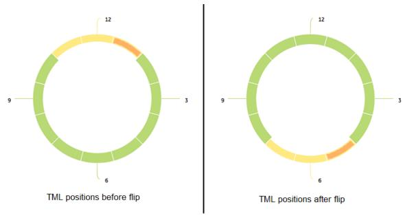
The following table illustrates the band positions for center and mirrored bands before and after a flip for an elbow with 12 band positions.
