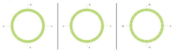
For example, in a piping component, if each band contains 4 TMLs, you can select a configuration of 4 positions. In this configuration, 4 equally spaced reference points (that is 3, 6, 9, and 12) are available along which the component can be rotated. The reference point for rotation is the Top Center. In this example, position 12 is the Top Center.
