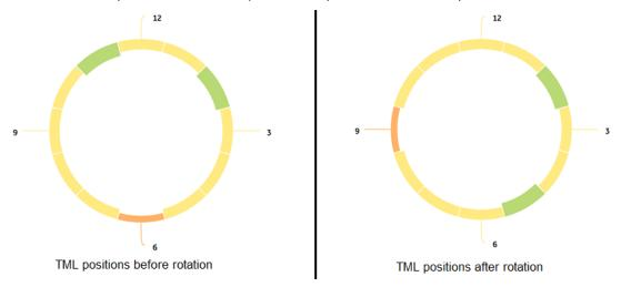
After a spool is rotated, the corrosion analysis for each TML within the bands is re-calculated based on the corrosion rate at the new position. This results in an updated remaining life for the component.
