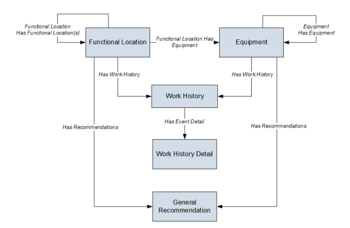
**Note:** In the diagram, boxes represent entity families and arrows represent relationship families that are configured in the baseline database. You can determine the direction of each relationship definition from the direction of the arrow head: the box from which the arrow originates is the predecessor, and the box to which the arrow head points is the successor.
