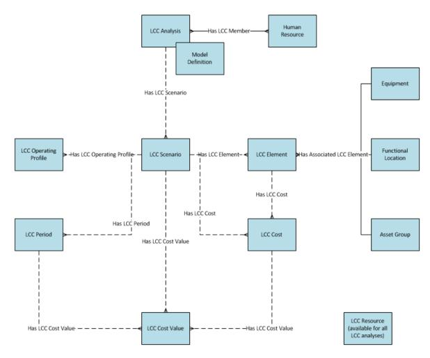
**Note:** In the diagram, boxes represent entity families and lines represent relationship families that are configured in the baseline database. You can determine the direction of each relationship definition from the direction of the arrowhead: the box from which the arrow originates is the predecessor, and the box to which the arrow head points is the successor.
