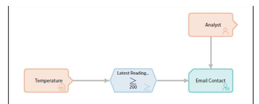
In this example model, the node named Temperature is an OT Connect Tag node which represents a process historian tag. When this policy is executed, if the Latest Reading Value that is associated with the process historian tag is greater than or equal to 200, the GE Digital APM system will send an email message to the email address that is specified in the Human Resource record that is associated with the Analyst User node.
