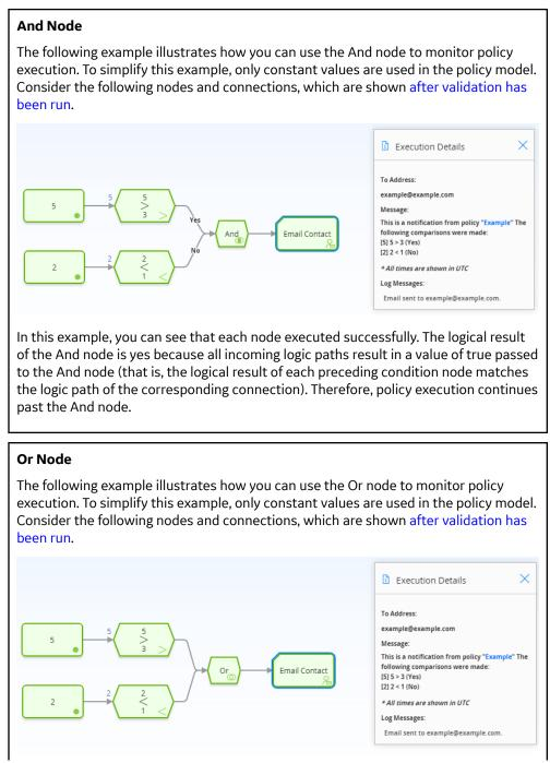
In this example, you can see that each node executed successfully. The logical result of the Or node is yes because the logical result of at least one incoming logic path results in a value of true passed to the Or node (that is, the result of the 5 > 3 Condition node is yes, which matches the logic path of the corresponding connection). Therefore, policy execution continues past the Or node.
