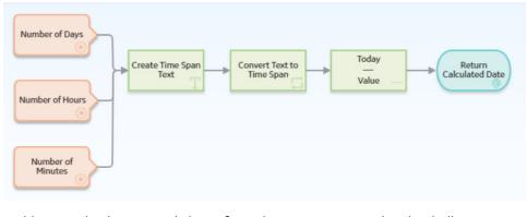
In this example, the Text node is configured to create a text string that indicates a time span, using the values represented by the Point Value nodes. Because the Subtract node cannot perform any calculation on a text string, the Convert Type node converts the string to a value of the Time Span data type. The converted time span value is then used in the Subtract node to calculate the required date.
