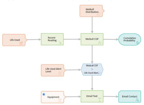
The threshold percentage of life used for the equipment is stored as a Technical Characteristic. The life data of the equipment (for example, hours for turbine, starts for crane, take-offs for aircraft, tonnes moved for mining equipment), is stored as Measurement Location readings.
