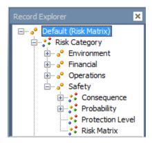
3. Below the *Safety* node, right-click the *Protection Level* node, and click **Create a** new Protection Level to link to Safety.
