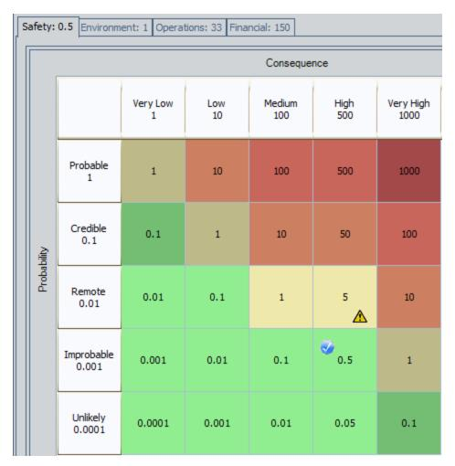
After you have selected a value on each tab, the selected values are used in a calculation to determine the overall risk rank.
