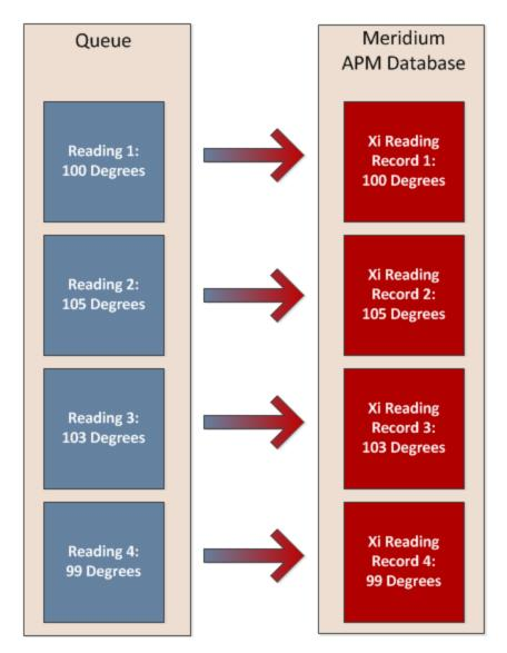
Now, suppose that the Process Data Integration Service runs again and finds an additional two readings. In this case, the two new readings are transferred to your Meridium APM database. Also, because you configured the system to store only two readings, all four Xi Reading records representing the previous four readings are deleted automatically. This scenario is illustrated in the following image.
