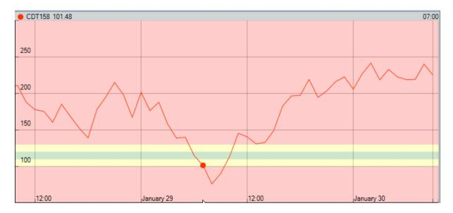
Finally, if you point further to the right, you can see that the reading value increases to *140.54*, which falls within the red shaded regions, which represents an Alert reading status.
