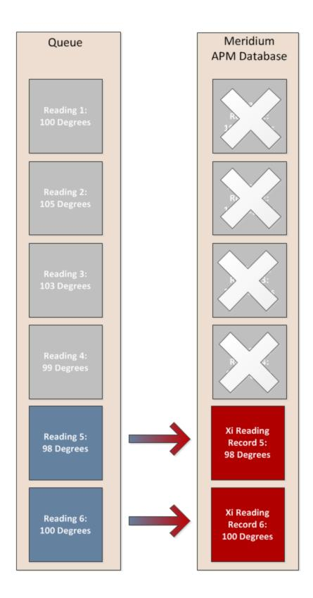
Finally, suppose that the Process Data Integration Service runs once more and finds one more new reading in the queue. In this case, that new reading will be transferred to the Meridium APM database as an Xi Reading record, and one Xi Reading record will be deleted automatically so that the Meridium APM database always contains only the two most recent readings. This scenario is illustrated in the following image.
