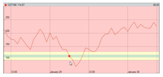
In this example, the reading value is *114.87*, which falls within the green shaded region, which represents a Normal reading status.
