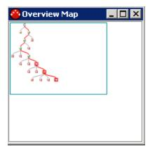
The Logic Tree appears in a box in the upper left corner of the **Overview Map** window. The box that appears around the Logic Tree indicates the scope of the area that is currently magnified in the diagram canvas. You can move the magnifying box to various locations on the tree and the diagram canvas will display that portion of the tree.
