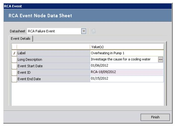
Each RCA Analysis will have one Failure Event node, which will always appear at the root level of the <u>Logic Tree hierarchy</u> and as the first node in the <u>Event Diagram</u>. For example, the following image shows the Failure Event node as it appears in the Logic Tree in our <u>Cooling Water Pump example</u>.
