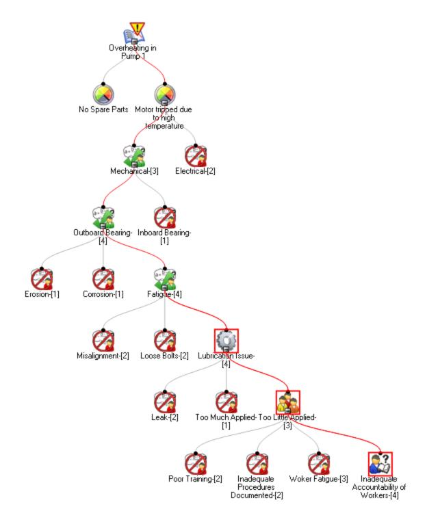
In this case, the root cause for the pump failure would be identified as *latent* (i.e., inadequate accountability of workers), which lead to *human* (i.e., too little applied) and *physical* (i.e., lubrication issue) causes. Now that a hypothesis has been verified and the root cause has been determined, you can create RCA Recom-
