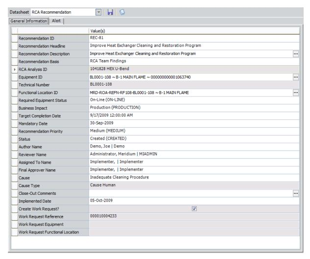
After the recommendation is completed, the value in the Status field of the RCA Recommendation record can be marked as *Implemented*. The success of the implemented
