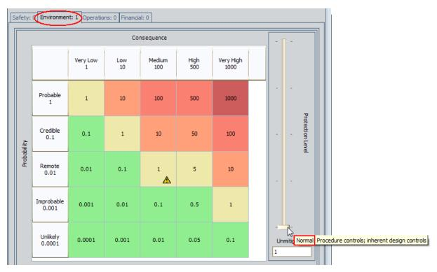
In this image, you can see that the Protection Level Definition name is *Normal*, and the description is *Procedural controls; inherent design controls*. You can also see in the **Unmitigated** cell (below the slider) that the factor for this Protection Level Definition is *1*. In this case, any number that is selected on the **Environment** tab will be multiplied by 1 to determine the total risk value for the Environment risk category.
