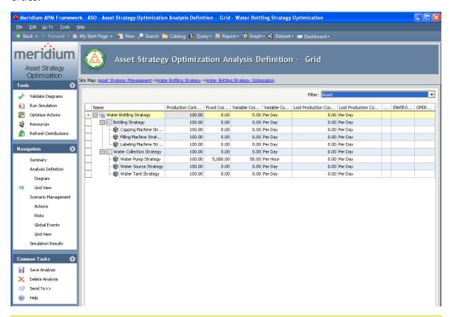
Note: The Asset Strategy Optimization Analysis Definition - Grid page displays Asset, Buffer, Distribution, Link, Risk, Subsystem, and Switch elements. Sensor elements can be viewed only on the Asset Strategy Optimization Analysis Definition - Diagram page.
