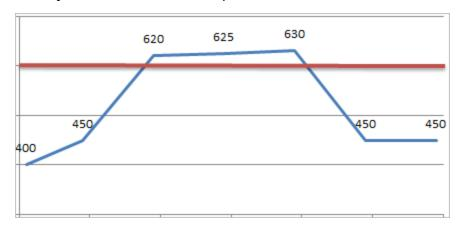
Here, you can see that the first reading value that exceeded the threshold value is 620. After that, two consecutive reading values also exceeded the threshold: 625 and 630. These additional reading values, however, are not treated as a second occurrence of exceeding the threshold value because they are consecutive. Therefore, the condition Count > 1 would be false and the condition Accumulated Time > 3 Days would be true.
