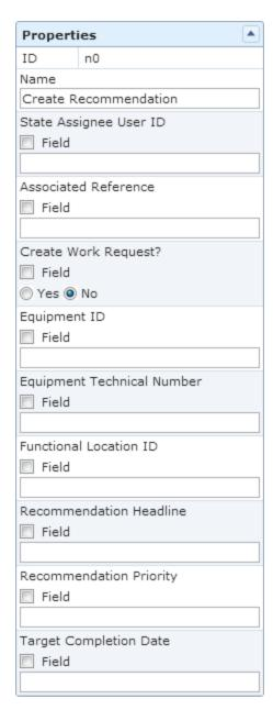
The **Properties** window for a Create Recommendation node contains the items that are described in the following table. You will use the <u>Field check box and subsequent</u> <u>options</u> to define the values in each section. The values that you define in each section will be used to populate the corresponding fields in the <u>Policy Recommendation record</u> that is created.
