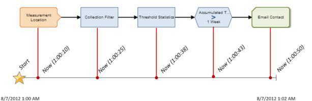
You can see from this image that the policy execution begins at 1:00 A.M. The first node, *Measurement Location*, is executed at 1:00:10 A.M. The second node, *Collection Filter*, is executed at 1:00:25 A.M., and so on.
