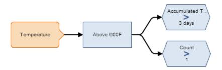
In this diagram, the *Temperature* Xi Tag node is connected to the *Above 600 F* Threshold Statistics node, which is also connected to two Greater Than nodes: *Accumulated Time > 3 Days* and *Count > 1.*
