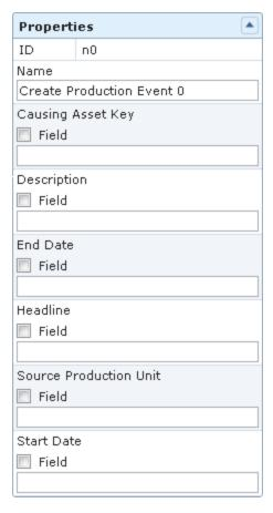
The **Properties** window for a Create Production Event node contains the items that are described in the following table. You will use the <u>Field check box and subsequent</u> <u>options</u> to define the values in each section. The values that you define in each section will be used to populate the corresponding fields in the Production Event record that is created.
