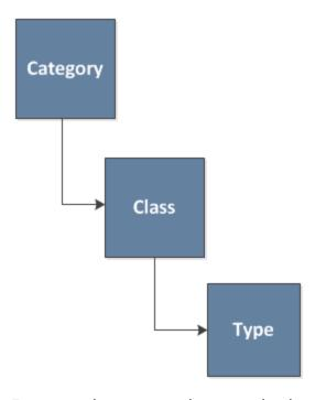
For example, suppose that your database contains many Equipment records representing pumps, some of which are centrifugal pumps and some of which are reciprocating pumps. Rather than classifying them all as simply *pumps*, you would want to classify them according to the levels defined above. So, you might end up with a classification like the one shown in the following image.
