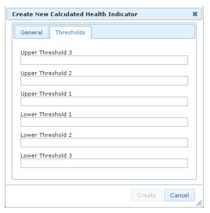
14. Type values in the threshold text boxes to indicate the thresholds against which values that are defined for this health indicator (that are stored in Health Indicator Value records) will be compared. For example, if Health Indicator Value records that are linked to this Health Indicator record will store a numeric value representing an overall health index on a scale of 1 to 10, where 1 represents critical health and 10 represents excellent health, you might define the thresholds like this:
