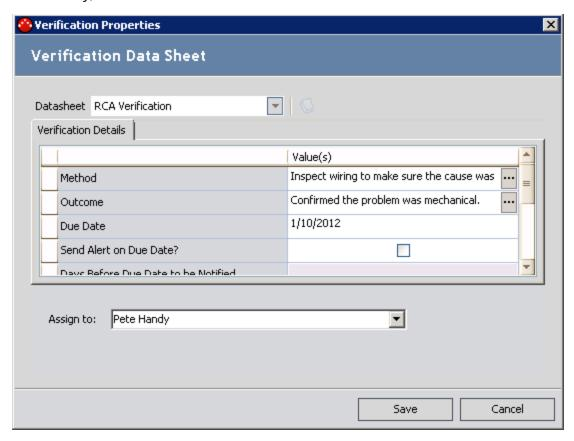
The task defined in this RCA Verification record instructs Pete Handy to inspect the wiring for the cooling water pump to ensure that the problem was not electrical, but mechanical.
