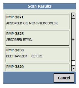
The **Scan Results** screen displays a list of checkpoints returned by the scan. Asset information is displayed for each checkpoint in the list. Specifically, the following values from the corresponding Measurement Location record are displayed for each checkpoint:
