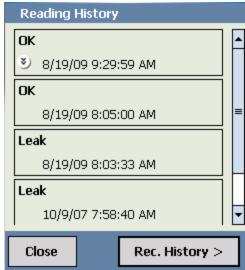
The **Reading History** screen displays a log of recent Readings that are linked to the Measurement Location. Note that it displays only the Reading records that have been uploaded to Meridium APM. In addition, the device will display only readings that have been completed, ignoring any *Non-compliant*or*Ignored*readings. By default, the screen displays the last five Reading records that were linked to the Measurement Location record.
