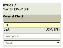
If, however, you change the reading value from 30 to 40, a message will appear indicating that the reading value must be lower than 35, and the reading value will be reverted back to 30 automatically.
