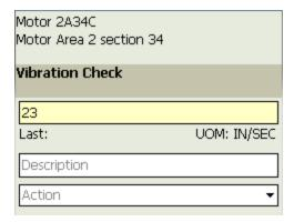
5. In the **Desc** text box, enter comments about the reading or the condition of the piece of equipment or location being inspected.
