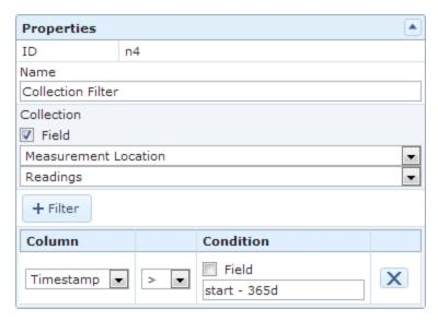
Alternatively, if the Collection Filter node included a start time of *now - 365d*, as shown in the following image, the Meridium APM system would evaluate values beginning with 1:00:25 A.M.
