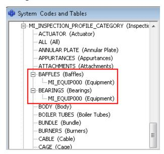
Notice how the referenced System Codes use the ID *MI\_EQUIP000*, which is the family ID of the Equipment family.
