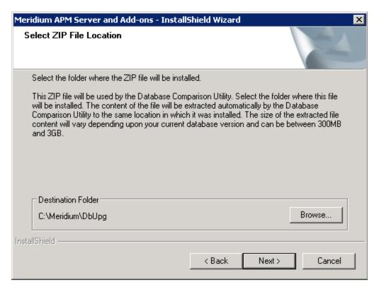
The **Select ZIP File Location** screen lets you specify the location where you want the ZIP file of database content to be installed. This ZIP file is used by the Database Comparison Utility. By default, the ZIP file will be installed in the folder **C:\Meridium\DbUpg**. You can, however, select a different location.
