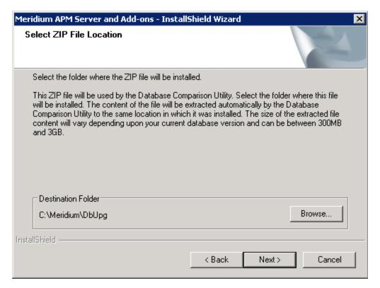
The **Select ZIP File Location** screen lets you specify the location where you want the ZIP file of database content to be installed. This ZIP file is used by the Database Comparison Utility. By default, the ZIP file will be installed in the folder **C:\Meridium\DbUpg**. You can, however, select a different location.
