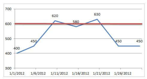
In the graph, you can see that the process historian recorded a reading value above 600 *two* times, where one value was 620 (on 1/10) and the other value was 630 (on 1/20). These values are treated as two separate occurrences of exceeding the threshold value because the reading value actually dropped below 600 between those two dates. In this scenario, the condition *Count* > 1 would be true, but the condition *Accumulated Time* > 3 *Days* would be false.
