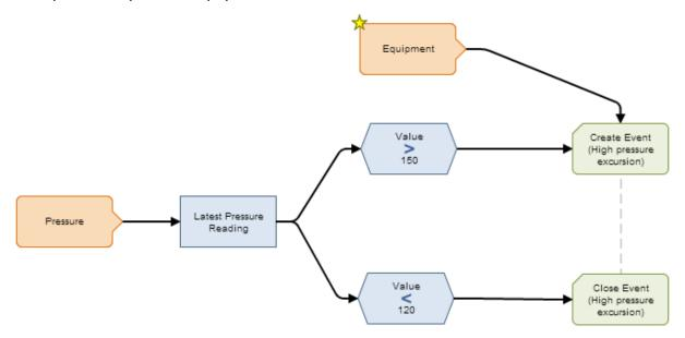
The *Equipment* node has been identified as the primary node, as indicated by the yellow star that appears on the top left corner of the node in the diagram.
