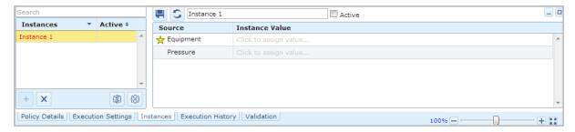
Because you have specified the Equipment node as the primary node, a yellow star appears to the left of the node name in the **Source** column. For this node, you will need to <u>specify the primary record</u>, (i.e., the Equipment record). In the following image, the Equipment record with the Record ID ~ #1 STEAM REHEATER ~ HXST 130 has been specified.
