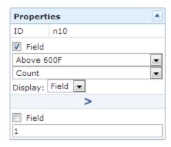
As shown in the following image, you can use the **Properties** window for the *Accumulated Time > 3 Days* Greater Than node to select the input *Accumulated Time* from the Threshold Statistics node.
