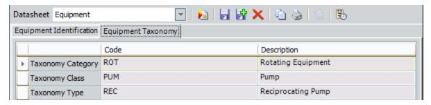
...based upon the value *ROTPUMREC* in the Object Type field (shown on the datasheet as *Equipment Type*):
