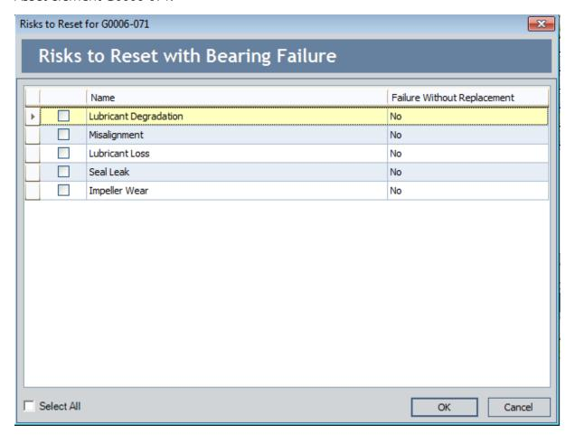
In this image, you can see that the **Risks to Reset** grid displays the Risks that are defined for the Asset element *G0006-071*. You can select these Risks to specify that the *Bearing failure* Risk (i.e., the source Risk) should reset additional Risks in the simulation.
