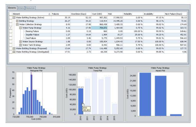
If desired, while viewing the Total Cost Trend graph, you can modify the graph to display the cost trend for each cost type that is included in the selected Scenario (i.e., Unmitigated, Proposed, or Active). To do so, below the x-axis, select the **Cost Type** option. Additionally, you can modify the graph to display the cost trend for each Risk that is included in the selected Scenario. To do so, below the x-axis, select the **Each Risk** option.
