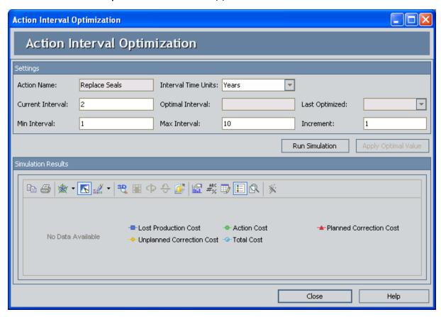
In this image, the **Action Interval Optimization** window displays the data necessary to optimize the Replace Seals Action.
