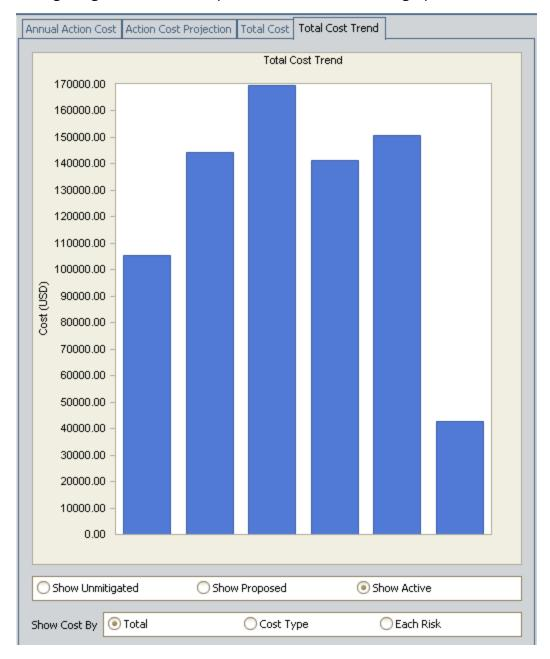
The Total Cost Trend graph in ASM displays the average (across all iterations) total cost of each Scenario for each analysis year or month, as defined by the value in the Time Analysis Type field in the root System Analysis record. If the Time Analysis Type field is set to:
