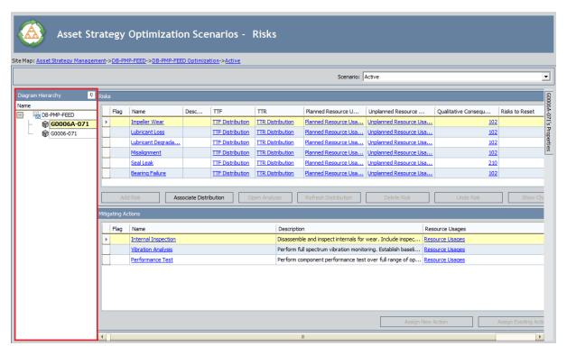
When you select an element in the **Diagram Hierarchy** pane, the associated Risks for that element are displayed in the **Risks**pane. For example, in this image, the selected *G0006A-071* Asset element has six associated Risks:
