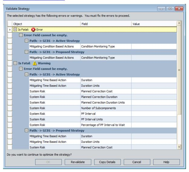
The window contains a grid, where each row represents a field that is used to yield simulation results but is missing a value. Each row represents a field in an Action record or a Risk record.
