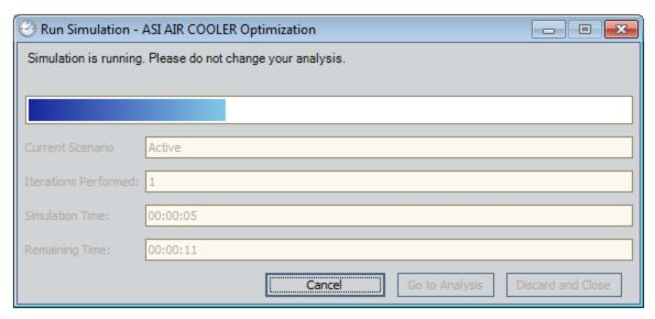
After the progress bar reaches the end, the **Go to Analysis** and **Discard and Close** buttons become enabled. If you do not want to view the results, you can click the **Discard and Close** button to close the **Run Simulation** dialog box. These instructions assume that you want to view the results.
