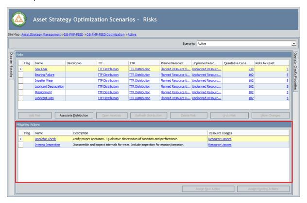
When you select a Risk in the **Risks** pane, the associated Actions for that Risk are displayed in the **Mitigating Actions** pane. For example, in this image, the *Seal Leak* Risk has two associated Actions: *Operator Check* and *Internal Inspection*.
