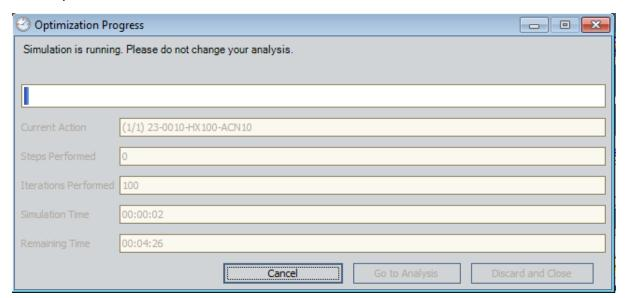
After the progress bar reaches the end, the **Go to Analysis** and **Discard and Close** buttons become enabled. If you do not want to view the results, you can click the **Discard and Close** button to close the **Run Simulation** dialog box. These instructions assume that you want to view the results.
