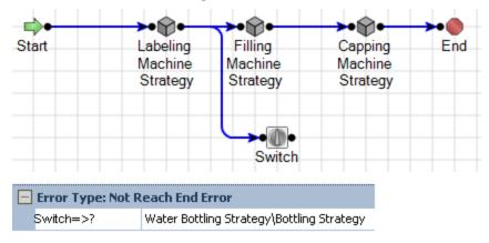
**Note:** This broken connection did not produce a Not Reach Start error because there is a complete connection from the End element to the Start element.
