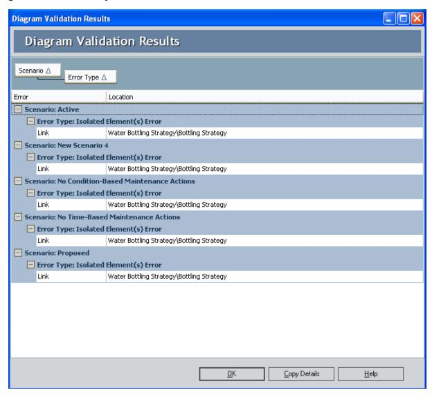
The **Diagram Validation Results** dialog box displays the **Error** grid, which displays error information, organized first by Scenario and then by error type.
