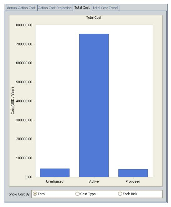
The Total Cost graph in ASM displays the average (across all iterations) total cost of each Scenario for the entire simulation period.
