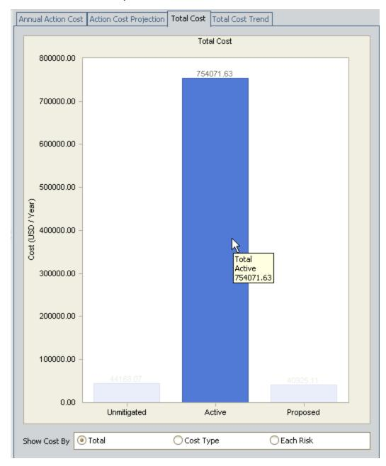
If you were to view the simulation results in the ASO Analysis that includes the Water Pump Strategy, you would see this same information. Specifically, in the **Elements** grid, you could view the value in the **Cost (USD)** column for the Active Scenario and the Water Pump Strategy element. The cost would be the same: \$754,072. You can see this value highlighted in blue in the following image.
