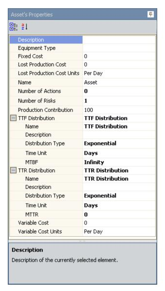
The **Properties** pane works much like a standard datasheet, where you can place your cursor in a cell and then modify the value for the associated field. If a value already exists in a field, it will be displayed in the appropriate cell. At the bottom of the **Properties** pane, any help text defined for the selected field will be displayed. For example, in the preceding image, the help text defined for the Description field is *Description of the currently selected element*.
