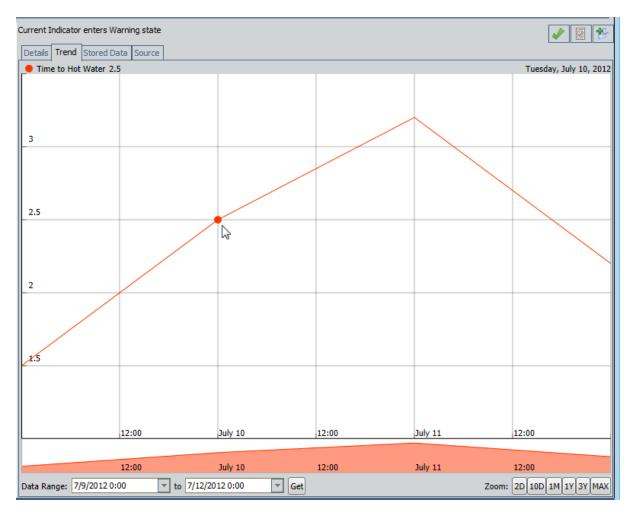
Below the graph, you will see another secondary graph with identical dates and times. This secondary graph allows you to shrink or expand the main graph to display only the portion that you want to see. When you pause on this secondary graph, your pointer appears as **4.** You can drag the left or right border of the secondary graph to emphasize a given area, as shown in the following image.
