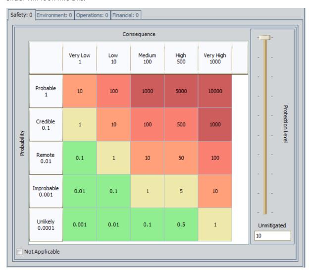
In this image, you can see that the highest level of the slider is selected (with the factor of 10), causing the value in the selected cell to be 50 (the result of the calculation 1 x 5 x 10, where 1 is the selected consequence and 5 is the selected probability). You can also see that the tooltip displays the default name and description as a concatenated value, *Default: Default*.
