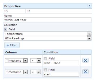
In the bottom grid, you can see the columns that you can use to filter data based on dates and times.
