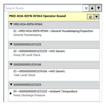
If a Measurement Location or Checkpoint Condition record is linked to one or more successor records, in the Route pane, an arrow will appear to the left of that Measurement Location or Checkpoint Condition node. The direction of the arrow indicates whether the successor nodes are displayed or hidden. You will see the following arrows in the Route pane:
