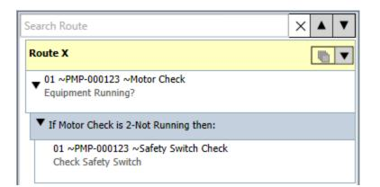
In this case, the condition statement is: *If Motor Check reading value is 2-Not Running, then display the Check Safety Switch checkpoint*. Further, you can define additional conditions for the:
