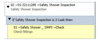
In this example, the final condition statement is: *If the Safety Shower Inspection is 2-Leak, then display the Check fittings checkpoint.*
