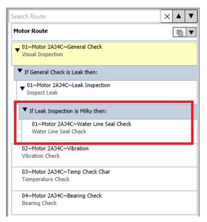
On the device, if the user identifies a milky leak as a result of performing the *Inspect Leak* checkpoint, the full list of checkpoints would look like this, where the *Water Line Seal Check* checkpoint has been inserted to account for this condition:
