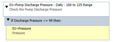
In this image, you can see that the final condition statement is: *If the Check the Pump Discharge Pressure reading is less than or equal to 99, then display the Pressure checkpoint.*
