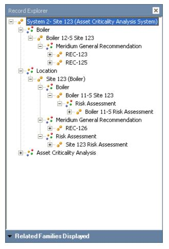
In the previous image, you can see the same relationships in a similar format in which you see them in the **Asset Criticality Analysis Systems** grid. For example, Boiler record *Boiler 12-S Boiler 12-S Site 123* is linked to TWO Meridium General Recommendation records: *REC-123* and *REC-125*.
