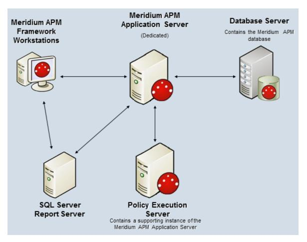
The following image provides an illustration of the architecture components that are required for deploying Policy Manager, including Process Data Integration.
