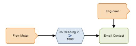
In this example diagram, the node named *Flow Meter* is an Xi Tag node which represents an Xi Tag record. When this policy is executed, if the DA Reading Value that is associated with the Xi Tag record is greater than 1000, the Meridium APM system will send an email message to the email address that is specified in the Human Resource record that is associated with the *Engineer* User node.
