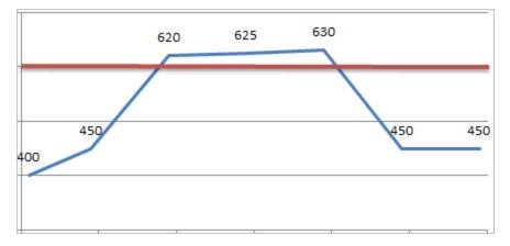
Here, you can see that the first reading value that exceeded the threshold value is 620. After that, two consecutive reading values also exceeded the threshold: 625 and 630. These additional reading values, however, are not treated as a second occurrence of exceeding the threshold value because they are consecutive. Therefore, the condition Count > 1 would be false and the condition Accumulated Time > 3 Days would be true.
