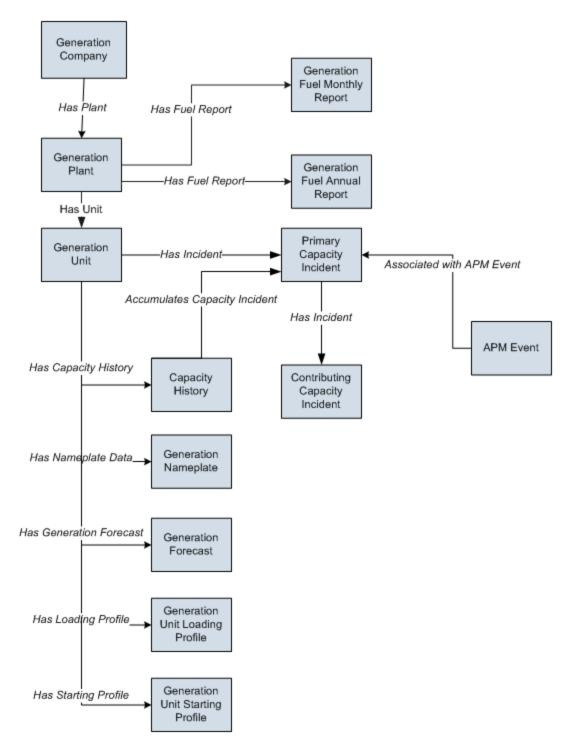
This figure shows only one box for the Generation Nameplate family. The Generation Nameplate family contains the following subfamilies, each of which is related to the Generation Unit family through the Has Nameplate Data relationship:
