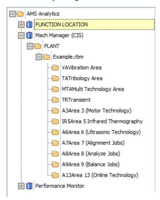
**Note:** One AMS Analytics data source node will exist in the tree for each *enabled* AMS Asset Data Source record that exists in the Meridium APM database.
