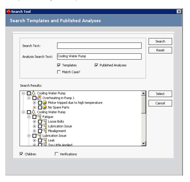
In this image, because the text Cooling Water Pump appears in the Analysis Search Text text box, the search results display the published RCA Analysis Cooling Water Pump and the hierarchy beneath it. The hierarchy displays:
