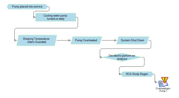
3. Diagram each failure mode in detail. For this example, you would create a Logic Tree like the one shown in the following image.
