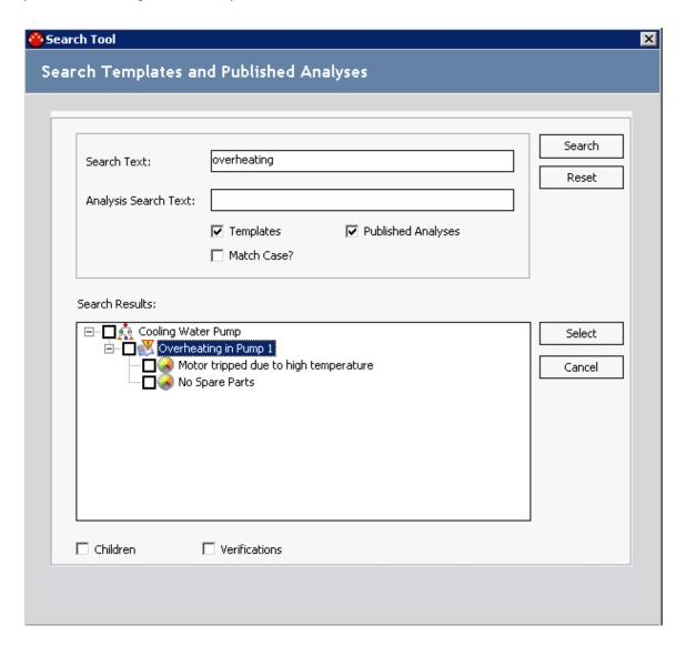
In this image, because the text *overheating* appears in the **Search Text** text box, the search results display the Failure Event Overheating In Pump 1. In addition, the hierarchy displays:
