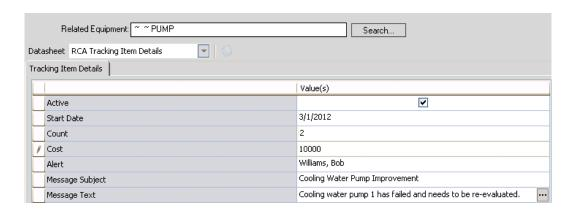
The value 2 in the Count field indicates that if the number of Failure records linked to the Equipment record *Pump* exceeds two, the alert email will be sent to Bob Williams. Note also that in the Cost field, the value 45 indicates that if the sum of the failure cost exceeds \$10,000, the alert email will be sent to Bob Williams.
