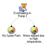
A given failure event can have multiple failure modes. For example, the image shows the failure modes from our Cooling Water Pump failure example. The Failure Event node (i.e., the overheated pump) is associated with the following Failure Mode nodes:
