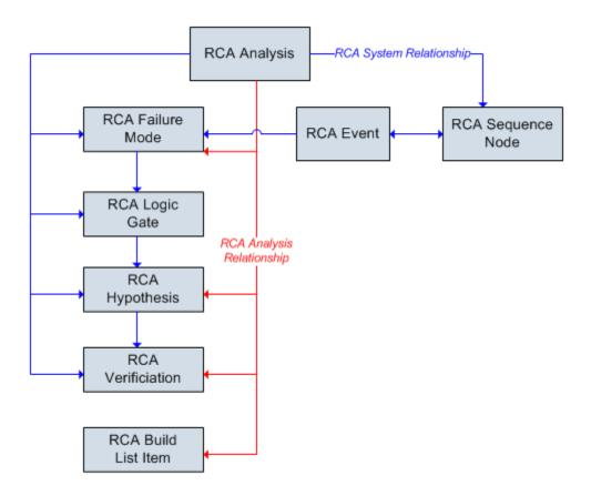
Records in the RCA Logic Gate family can be linked to other records in the RCA Logic Gate family. Additionally, records in the RCA Sequence Node family can be linked to other records in the RCA Sequence Node family.
