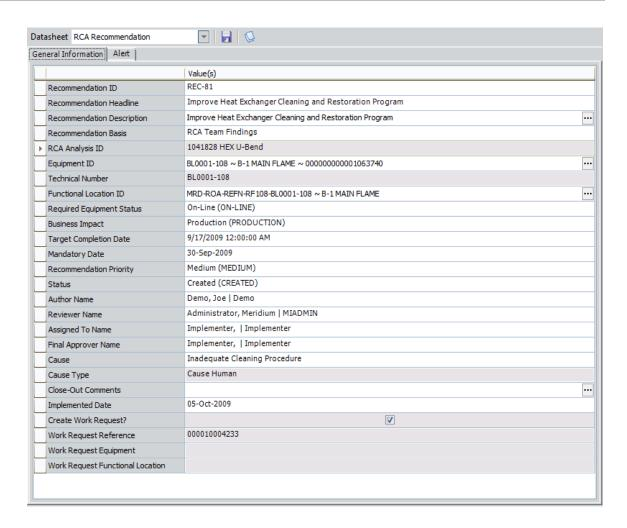
After the recommendation is completed, the value in the Status field of the RCA Recommendation record can be marked as *Implemented*. The success of the implemented recommendation, however, should continue to be tracked. If the piece of equipment or location continues to fail after the recommendation has been implemented, the RCA Recommendation record can be flagged for reevaluation.
