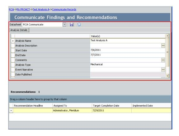
Note: When you access the Communicate Records page, the RCA Communicate datasheet is displayed by default. If desired, you can select a different datasheet in the **Datasheet** list to modify.
