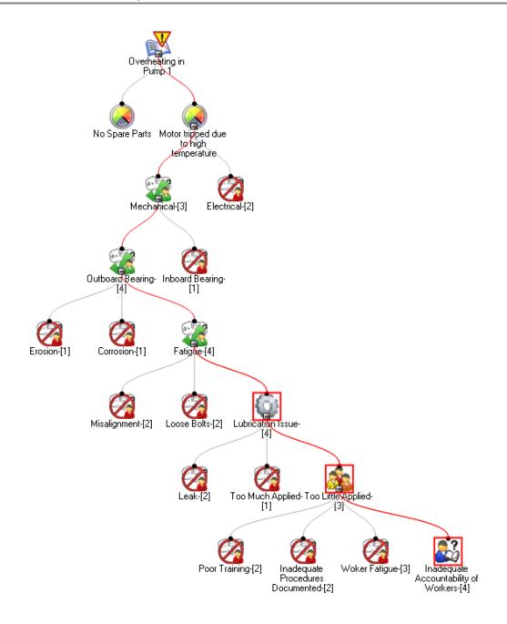
In this case, the root cause for the pump failure would be identified as *latent* (i.e., inadequate accountability of workers), which lead to *human* (i.e., too little applied) and *physical* (i.e., lubrication issue) causes. Now that a hypothesis has been verified and the root cause has been determined, you can create RCA Recommendation records to communicate your findings on how to prevent this failure in the future.
