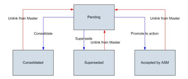
Note: The Promote to Action operation and Accepted by ASM states are included in the baseline State Configuration for the Reliability Recommendation family. The associated functionality will not be fully functional, however, unless the Asset Strategy Management module is active.
