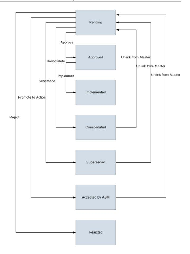
Note: The Promote to Action operation and Accepted by ASM states are included in the baseline State Configuration for the RCM FMEA Recommendation family. The associated functionality will not be fully functional, however, unless the Asset Strategy Management module is active.
