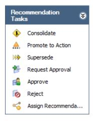
The Recommendation Tasks menu on the Recommendation Management page displays links that allow you to perform operations against a Recommendation record or set of Recommendation records. The links that are available depend upon the State Configuration that is defined for the Recommendation family and the current state of the selected Recommendation record(s).
