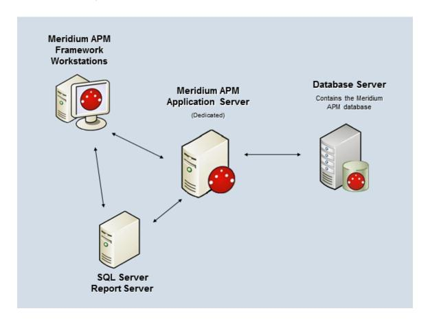
This image shows *one* dedicated Meridium APM Application Server. In a deployment where multiple dedicated Meridium APM Application Servers exist, connections can be managed manually by assigning users to specific servers, or they can be managed automatically by a hardware- or software-based network load balancer.
