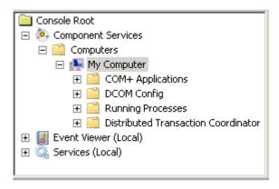
3. Expand the Distributed Transaction Coordinator node, and select Local DTC.
