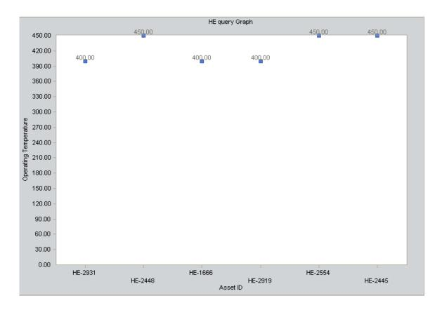
Suppose all of the records in this graph belong to the Shell and Tube Heat Exchanger family, and you order all Shell and Tube Heat Exchangers from the same manufacturer. You might want to create a new Shell and Tube Heat Exchanger record from this graph and populate the Asset Manufacturer field automatically with the manufacturer that supplies your Shell and Tube Heat Exchangers.
