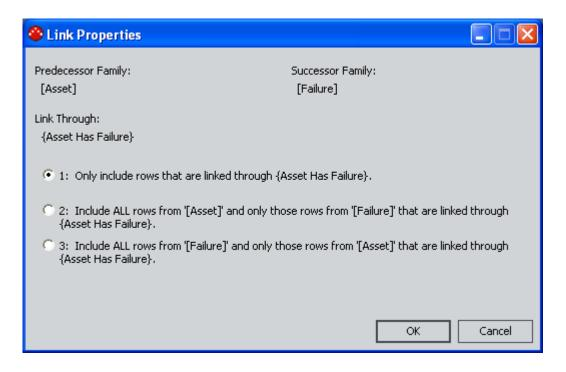
From the Link Properties window, you can determine the query source families, indicated by the labels Table #1 and Table #2. You can also determine the joined fields, which are listed in the Field #1 and Field #2 lists. In addition, you can determine if the join is an inner join, a left join, or a right join. An inner join is represented by the first option, a left join is represented by the second option, and a right join is represented by the third option.
