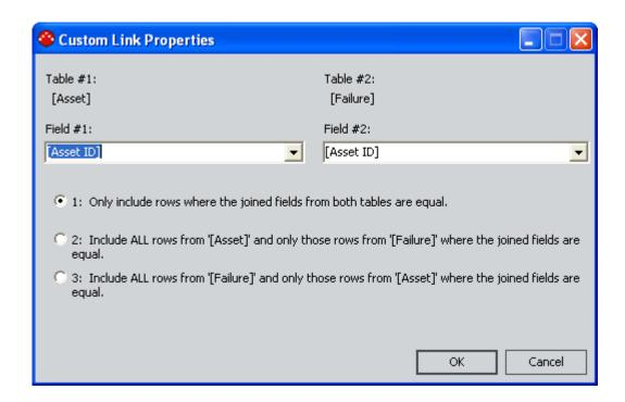
The names of Table #1 and Table #2 appear at the top of the dialog box. These table names represent the names of the selected query source families. The names of the join fields appear beneath the names of the families in the lists labeled Field #1 and Field #2. You can modify the selected fields by choosing a different selection from the Field #1 list or Field #2 list.
